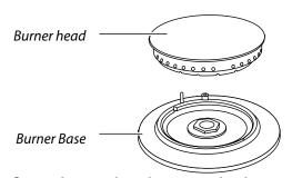
When fitting burner head, ensure this locates properly within the base.
